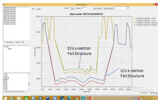
Fig.13. Cross-section at u/s and d/s of Fall-Structure- at RD-77 showing aggradation and degradation
